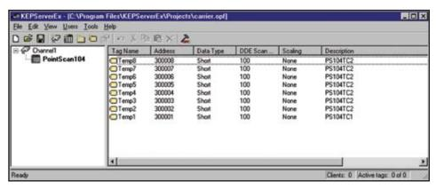
KEPServerEX software lets you use any DDE or OPC client application to collect data from IOtech's PointScan series distributed I/O modules
